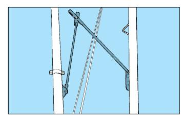
• Trolling and paravane stabilizer poles **must** have devices that lock the poles down and limit their downward travel. Unsecured poles that pop out of position can damage the vessel, make the boat unstable, or injure crew.
