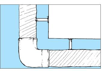
• Make sure all exhaust pipes are away from wood and other material that can catch fire. Cover the pipes with lagging where needed.
