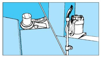
• To warn of flooding or high water levels, water-level sensors that sound an alarm **must** be installed in the engine room bilges and in the shaft log or the lazarette.
