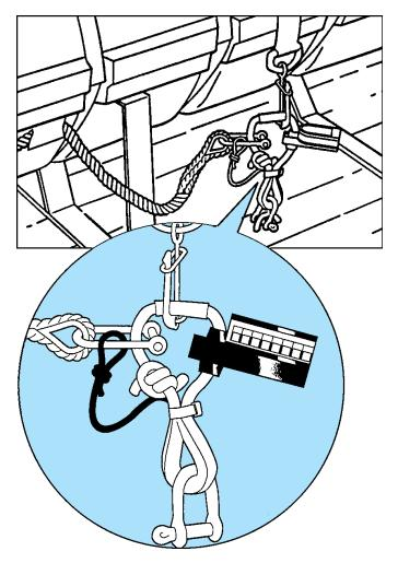
The proper installation of a hydrostatic release
