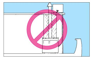
• Stove fuel tanks and lines **must not** be located directly above the stove. A leaking tank or line above the stove can easily catch fire.
