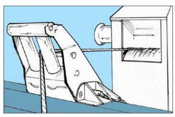
All movable davits **must** have a device to lock them in place so the davit does not jerk back and strike crew members. Don't use a bolt in place of a locking pin.
