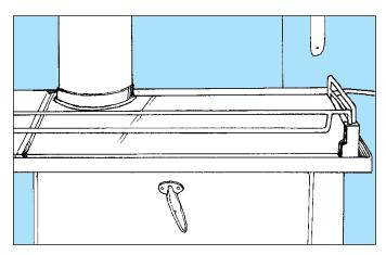
• Galley stoves **must** have guards to stop cooking gear from sliding off the stovetop.
