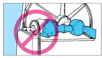
Moving parts of power-operated equipment such as chain and belt drives, gearing, and shafting—must be guarded to avoid allowing hands, hair, or clothing to be caught. (Equipment such as a capstan can't be guarded because of the way it operates.)
