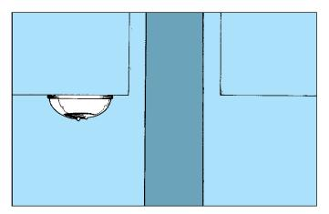
• A heat sensor that sounds an alarm **must** be installed near the engine exhaust.
