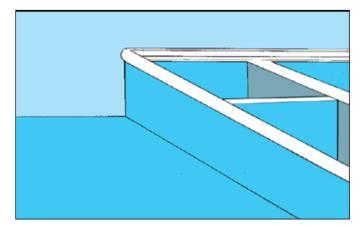
• Be aware of open tanks. Cover tanks after delivering or unloading fish. Secure them in heavy weather to keep water from sloshing out of the tanks. Water loss from the tanks can lead to free surface effect and related stability problems.
