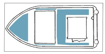
• Decks **must** have non-skid surfaces except where a smooth surface is needed for handling fish.
