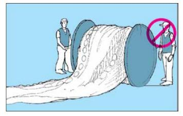
• Never stand forward of the drum when rolling the cod end onto the drum. If the cod end goes over the drum, it can land 2.4 metres (8 feet) or more ahead of the drum.
