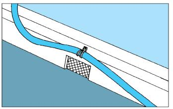
• Make sure scuppers are not blocked by equipment, tools, hoses, lines, or debris. Blocked scuppers can pose a serious hazard, especially in rough seas.
