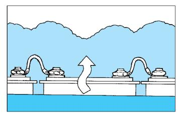
• Vent the battery storage area. Batteries give off toxic, explosive gas.
