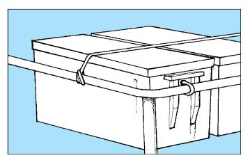
• Boxes for shrimp and fish **must** be secured with bolts, chains, tie-downs, and so on, to prevent them from sliding. If boxes slide, they can hit crew members or make the vessel unstable.
