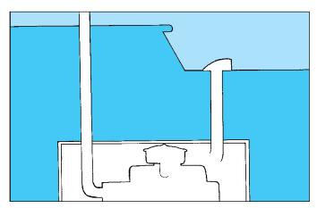
• Vent all closed spaces with gasoline engines. Exhaust gases or fuel vapours can be deadly if allowed to build up.
