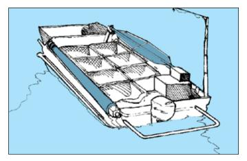
• Work areas on herring skiffs and punts **must** be arranged so crew members do not contact moving equipment such as beater bars and live rollers.
