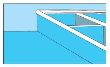
• Be aware of open tanks. Cover tanks after delivering or unloading fish. Secure them in heavy weather to keep water from sloshing out of them. Water loss from the tanks can lead to free surface effect and related stability problems.
