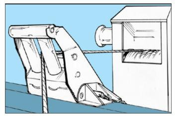
Pursing winches and davit leads must be positioned to ensure proper spooling of the line onto the winch drum. If the line isn't spooled properly—for example, if it spools only on one side of the drum—it is more likely to backlash when being let out. When gear spools properly, it eliminates the need for crew members to direct the line, and increases the life of the line by reducing damage to it.
