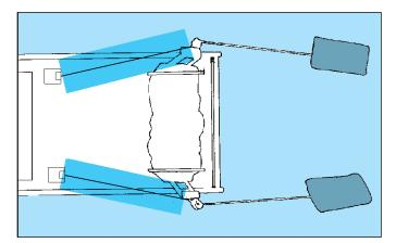
• Stay clear of the trawl warps when they are being set out. If a warp snaps, the line could strike a crew member.
