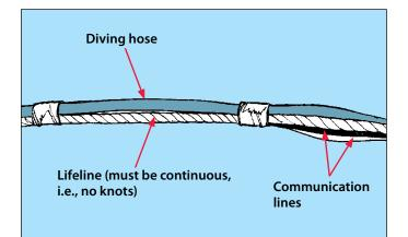
Surface-supply hoses must be a commercially manufactured twisted bundle or attached to lifelines to prevent undue stress on the supply hose or the helmet. Lifelines must be 16 millimetres (5/8 inch) in diameter, and made of polypropylene or other equivalent synthetic fibre. Divers must use only hoses designed and suitable for surface-supplied diving.
