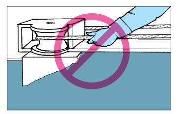
• Never handle a running line. Broken strands of wire rope can enter your hand and/or you may be pulled into a stationary block or other in-running nip point.
