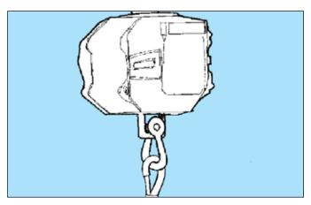
• Use a rated shackle or hook with a safety latch to attach the scale to the brailer. An open hook can slip, especially in heavy swells, causing the hook or the bag to hit crew members.
