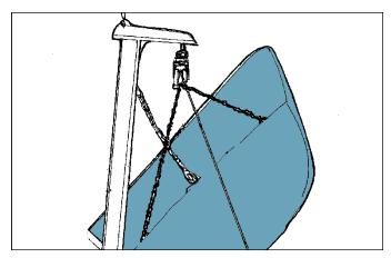
• When not being used, trawl doors and otter boards **must** be secured to davits.
