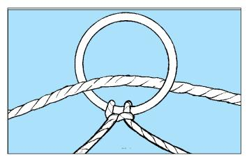
• Purse rings on seine nets **must** be secured to the middle of the ring strap. This prevents rings from falling and hitting crew when back hauling the net through the power block.
