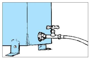
• Stove fuel tanks **must** have a shut-off valve at the tank. The valve allows you to turn off the fuel supply if there's a stove fire, if the stove controls break, or if the stove needs repair. Use proper fuel lines.
