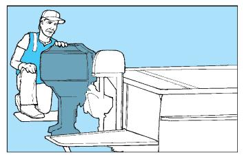
• Crew members **must** be taught how to safely clear fouled propellers on a herring skiff. Using standing grids, hoists, or tie-off lines can make clearing propellers safer.
