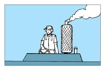
• In a power skiff, the exhaust system **must** be shielded to prevent burns and **must** direct exhaust away from the crew.
