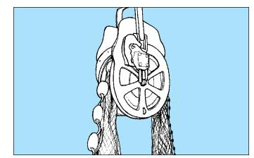
• When working on or fleeting the seine, power block operators **should** watch for and warn the crew of lead lines dropping from the block. Wear a hard hat whenever there is an overhead hazard.
