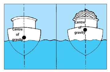
• Keep weight in the vessel as low as possible. This makes the vessel more stable and less likely to capsize. Make sure the vessel is not overloaded because overloading can cause the vessel to be unstable.
