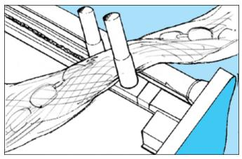
• Crew members **must** stay clear of stern spooling gear while it is operating. A major hazard is getting feet caught between the spooling roller cradle and the side of the boat. Add stop blocks to limit spooler travel to rails.
