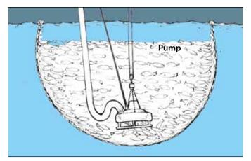
When seining for herring or sardines, pumping gear **must** be able to pump fish from the bottom of the bunt while the net is set. Dying fish create deadweight that can cause stability problems. Always carry enough extensions to pump the bunt of large sets.
