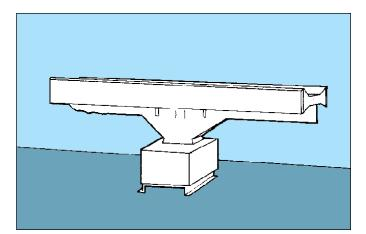
• Stay clear of the radar scanner. It can cause serious injuries when rotating. Put a "Do Not Operate Radar" sign on the wheelhouse radar when someone is working aloft.
