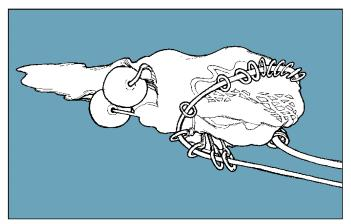
• All cod ends **must** have splitting straps so that fish can be dumped safely.
