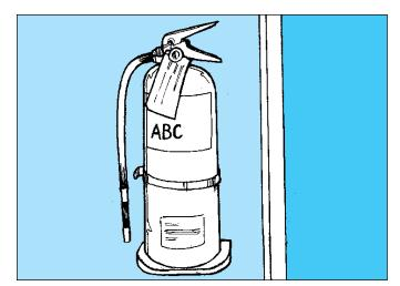
• Keep an ABC or AB fire extinguisher in the galley, near the entrance, if possible. Hang the extinguisher in a bracket, where it can be easily seen and reached.
