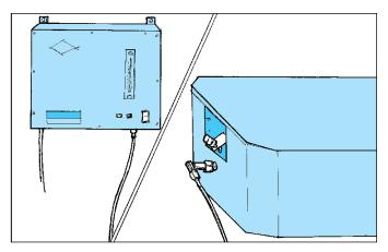
Follow the manufacturer's instructions, and check all hoses. They can become hard and cracked, causing leaks of ozone or pure oxygen from the concentrator. Leaks of oxygen can cause a fire or explosion.
