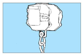
• Use a rated shackle or hook with a safety latch to attach the scale to the brailer. An open hook can slip, especially in heavy swells. When this happens, the hook or the bag can hit crew members.
