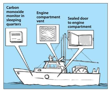
• To warn of possible carbon monoxide exposure, an audible marine grade carbon monoxide sensor, connected to an alarm system where practicable, **must** be installed in the crew quarters.
