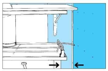
Galley stoves must be bolted down or otherwise secured so they don't slide or move. The space between the stove and the firewalls must be large enough to allow you to clean up oil and grease.
