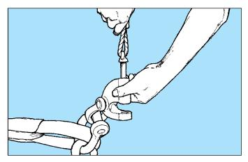
Inspect all end-of-net hardware for sticking blondies (quick-release shackles), worn straps, loose shackle pins, and other defects. Broken hardware can create unexpected hazards such as lines whipping and/or breaking, or equipment striking the crew.
