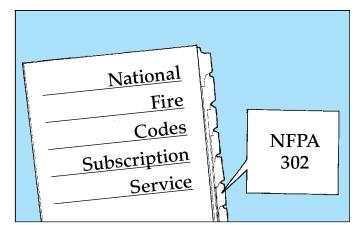
Be sure that installations for propane, compressed natural gas, and liquefied petroleum gas used for fishing vessel appliances are safe and in good repair. Such installations **must** conform to the most recent edition of National Fire Protection Association Standard 302: Fire Protection Standard for Pleasure and Commercial Motor Craft.
