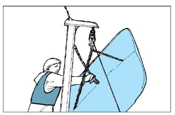
• Crew members **must** stay clear of the pinch points when hooking and unhooking the trawl doors from the davits. Serious injury will occur if a crew member is crushed between the doors and the side of the vessel.
