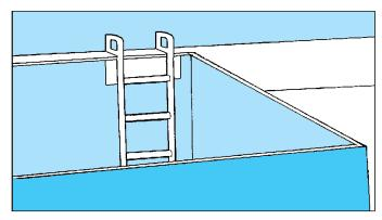
• For fish holds, use ladders that attach securely to the hold. If you need to use portable ladders, ensure they are tied off securely. Home-built ladders **must** comply with Part 13 of the Occupational Health and Safety Regulation.
