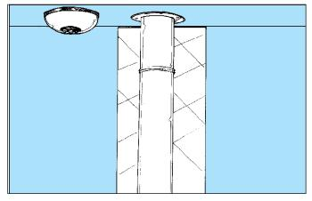
• A heat sensor that sounds an alarm **must** be installed above the stove or near the stove pipe.
