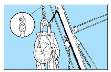
• Haul lines **must** be shackled to the power block. Use adequate shackles and regularly check their condition.
