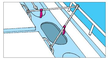
• Deck openings and hatches that need to be open for ventilation **must** be marked and guarded.
