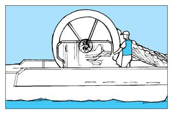
• The drum operator **must not** leave the controls while the drum is turning. Never attempt to remove the tow line hook or tuck the strap while the drum is turning. The drum operator needs to be able to stop the drum quickly in case of emergency. Consider hold-to-run controls.
