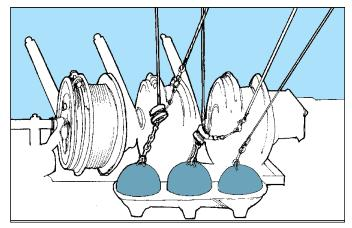
• Gurdy brakes **must** be kept in good working order. Crew **must** be able to stop the lines at all times.
