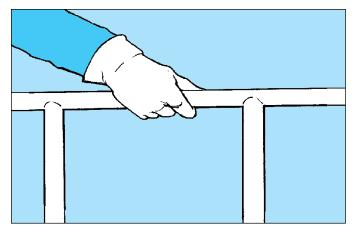
• Grabrails, handrails, or guardrails **must** be installed, where practical, to keep crew members from falling overboard.
