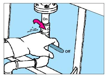
• When seacocks are not required to be open, turn the valve handle to the "off" position.
