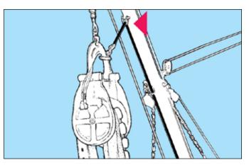
• Power blocks **must** be attached to an effective safety line when hanging above the deck.
