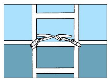
• Ladders **must** be of sound design and in good condition. When using portable ladders, they **must** be secured.
