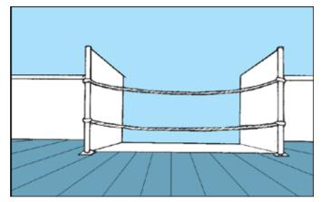
• Stern ramps **must** be roped off or guarded when not being used for trawling operations. If the ramps aren't guarded, crew members could accidentally fall down them.
