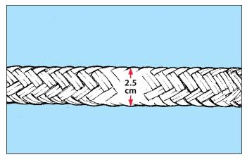
Power block haul lines must have a diameter of at least 2.5 centimetres (1 inch) of double braid nylon or the equivalent. The capacity of the line must be rated to safely secure power blocks. Inspect rope regularly, looking for wear, cuts, variations in sizes, and discolouration.
