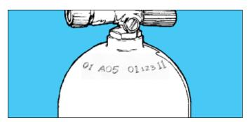
Scuba cylinders must be visually inspected internally every year. Cylinders must be hydrostatically tested every five years. Inspection and testing results must be documented in an equipment log book and must be available at the dive site. At a minimum, scuba divers **must** use the following equipment as appropriate to the diving conditions and as specified by the diving supervisor:
