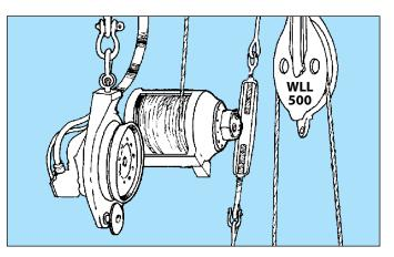
• All rigging—chains, slings, hoists, turnbuckles, derricks, blocks, and anchor gear—**must** be inspected prior to each use and kept in safe working order. Since chains are manufactured for different purposes, make sure the chain is designed for its intended use. Chains used for hoisting **must** be grade 80 or better.
