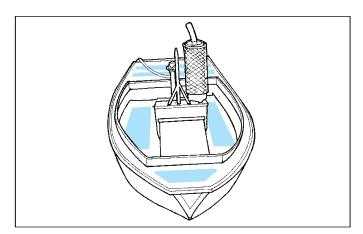
• Decks and floors **must** be non-skid, where practical, and the rails and sides of the skiff **must** be free of snags that can catch the net.
