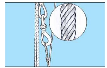
• Rigging including hooks **must** be inspected. Check the hardware, lines, and cables closely for signs of wear or stress. A worn or damaged hook **must** be replaced according to hook rejection criteria.
