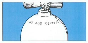
Scuba cylinders must be visually inspected internally every year. Cylinders must be hydrostatically tested every five years.
